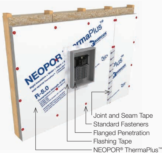
■ Figure 7: Typical Flanged Penetration (Vent, Box, etc.)
