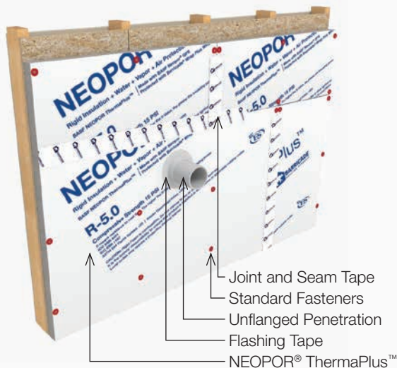
■ Figure 8: Typical Unflanged Penetration (Pipe, etc.)
