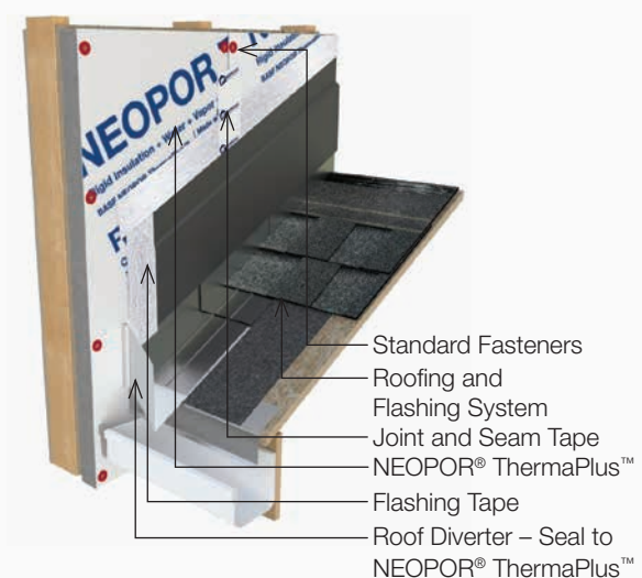
■ Figure 14: Typical Roof Diverter
