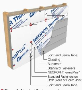
Figure 2: Standard Fasteners and Fastening Pattern
