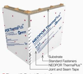
Figure 17: Typical Exterior Corner
