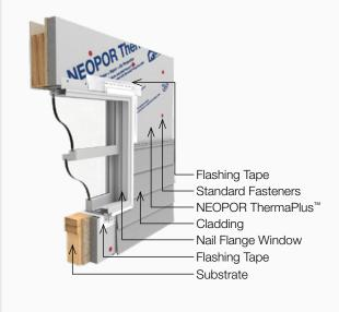
Figure 10: Typical Nail Flange Window
