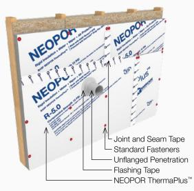
Figure 8: Typical Unflanged Penetration (Pipe, etc.)
