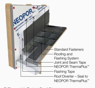
Figure 14: Typical Roof Diverter
