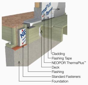
Figure 15: Typical Deck/Ledger
