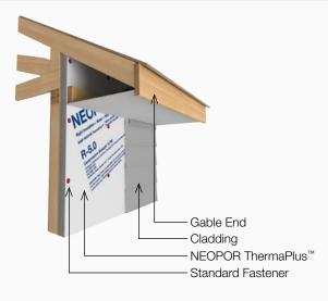
Figure 13: Typical Gable End/Top of Wall
