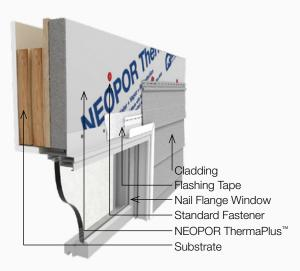
Figure 12: Typical Window Head (Jamb Similar) – Nail Flange Window
