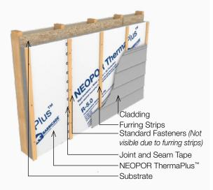
Figure 16: Typical Rainscreen Cladding on Furring Strips
