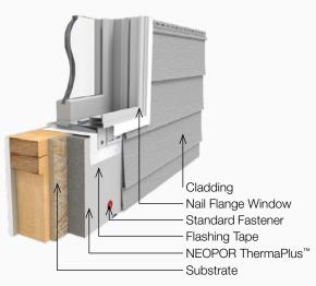
■ Figure 11: Typical Window Sill - Nail Flange Window
