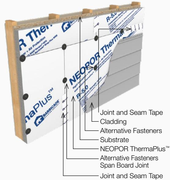
■ Figure 3: Alternative Fasteners and Fastening Pattern
