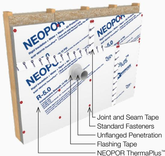
■ **Figure 8:** Typical Unflanged Penetration (Pipe, etc.)
