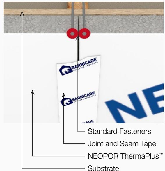
■ Figure 5: Joint and Seam Tape Covers Fasteners
