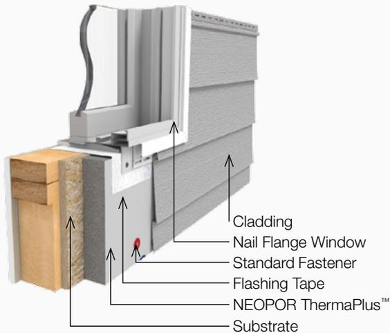
■ **Figure 11:** Typical Window Sill - Nail Flange Window
