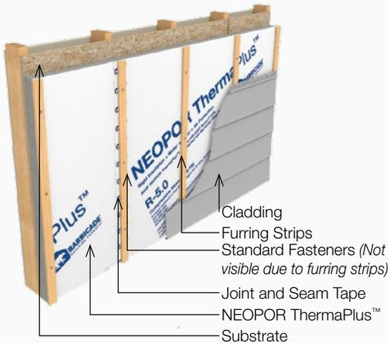
■ **Figure 16:** Typical Rainscreen Cladding on Furring Strips
