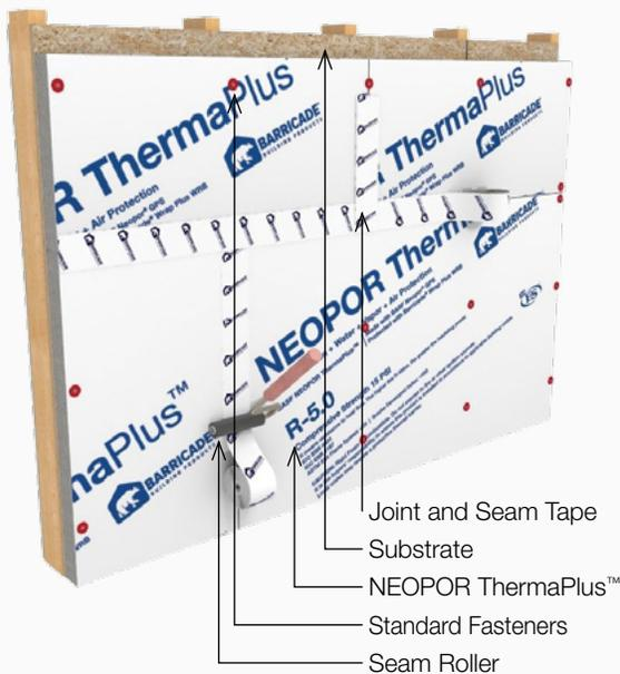
■ **Figure 6:** Typical Joint and Seam Tape Application
