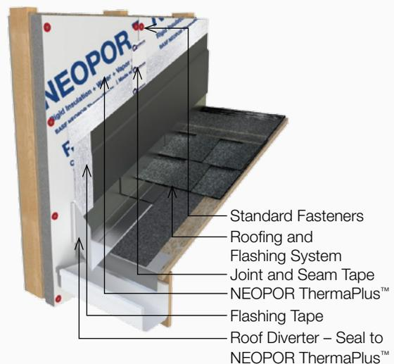
■ **Figure 14:** Typical Roof Diverter
