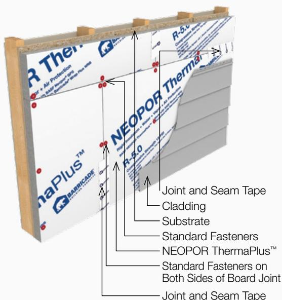
■ **Figure 2:** Standard Fasteners and Fastening Pattern
