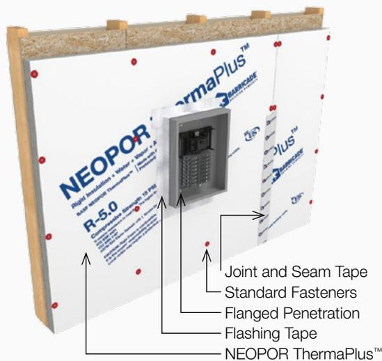
■ **Figure 7:** Typical Flanged Penetration (Vent, Box, etc.)
