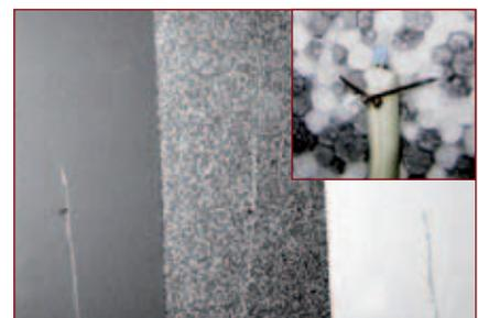
Insulation boards tested at the Fraunhofer Institute, with temperature sensors
