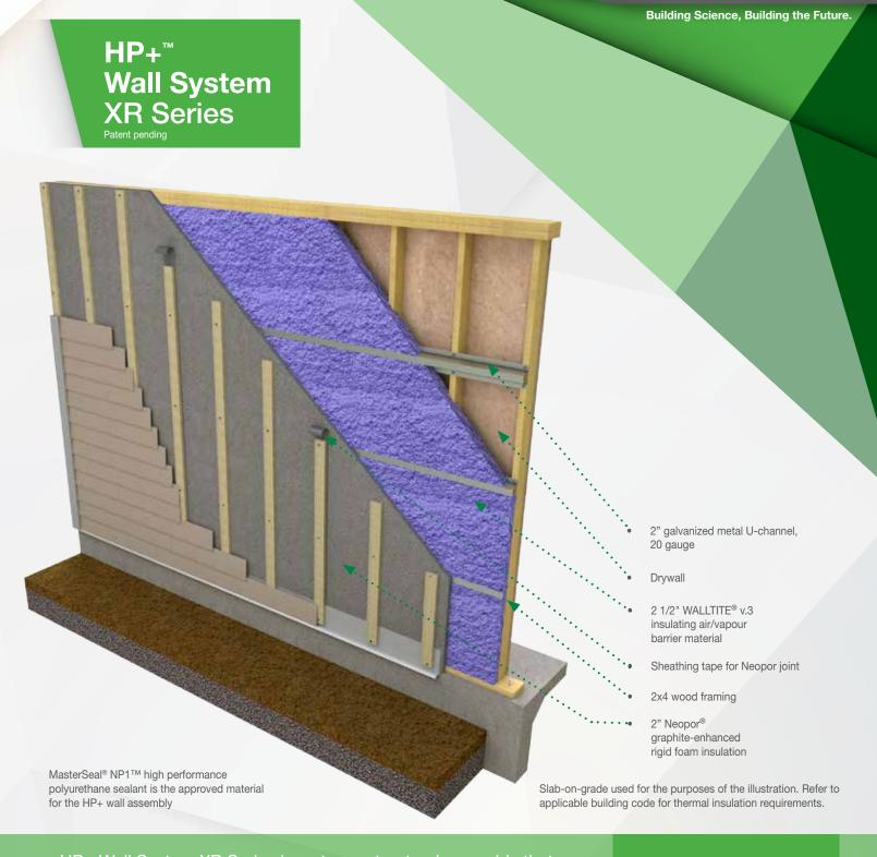
HP+ Wall System XR Series is a strong structural assembly that meets or exceeds building code requirements with a minimum nominal insulation R-value of R-25 up to R-45.8 with 2x4 wood framing. The XR Series offers exceptional energy and cost efficiencies.
