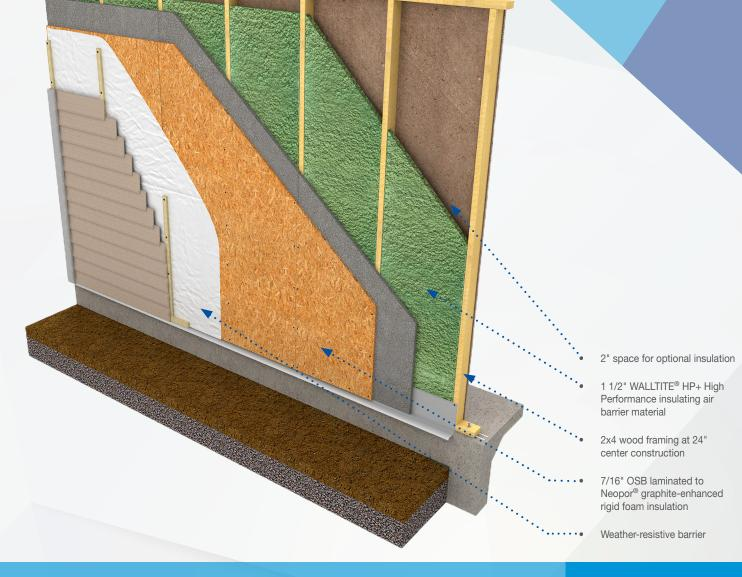
The HP+ Wall System X Series is a durable, structural assembly that offers additional durability for extreme design conditions like high wind zones and seismic zones. It meets or exceeds codes while using less wood than traditional construction, resulting in exceptional energy and cost efficiency.
