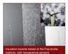
Additional tests at other institutes showed that at 4 cm below the surface of the white, mixed white-gray, and gray boards, the temperatures were nearly identical.
