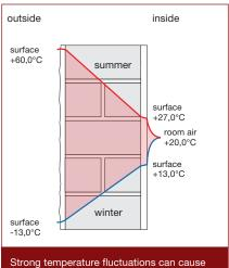
stresses and damages in the wall structure
