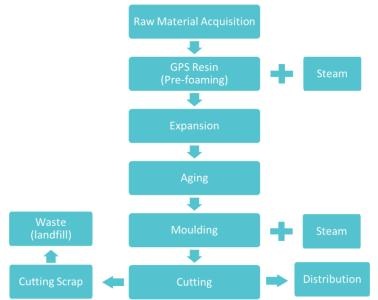
Figure 2: EPS Manufacturing Process
